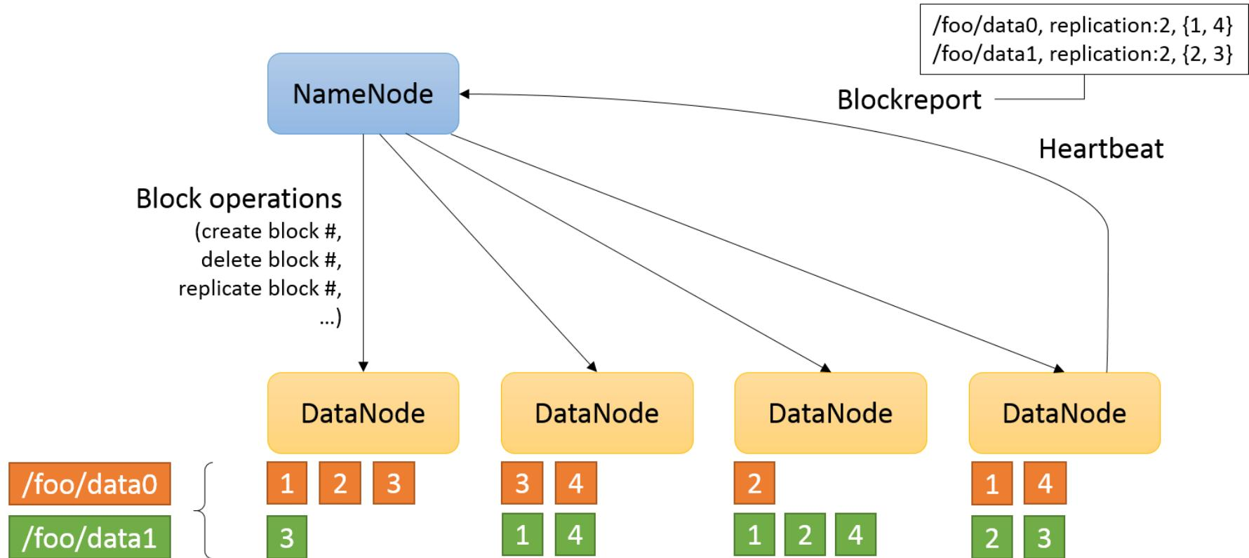
Each Datanode frequently (default, every 3 mins) sends a heartbeat and block report (list of available blocks) to the Namenode. If a Datanode does not send a heartbeat before `dfs.namenode.stale.datanode.interval` is reached, the Datanode is marked dead.
